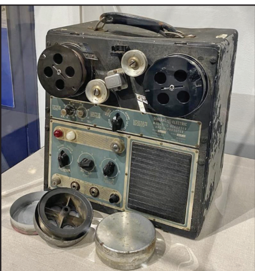
This wire recording and playback machine recorded tank, truck, artillery, and small arms sounds by pulling a 37 gauge steel wire over the recording head that magnetized each point along the wire to reproduce sound. The 3132nd Signal Service Company of the Ghost Army projected these sounds of combat towards the real U.S. Army in an attempt to disguise the U.S. Army in its locations and intentions, as well as draw enemy fire to keep them occupied in a certain area of the battlefield. This artifact, loaned from the National World War II Museum, is featured in the temporary Ghost Army exhibit at the ASOM through April 25, 2021.
