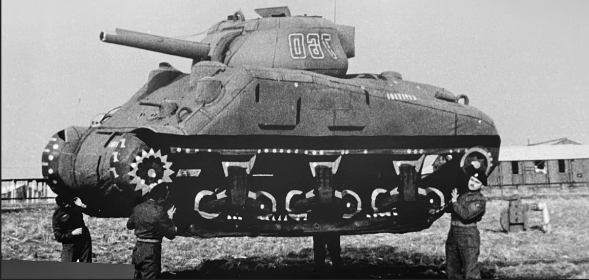
Ghost Army Soldiers lifting an inflatable tank. Built on a frame of inflatable tubes, the facsimiles were surprisingly realistic when viewed from a few hundred yards, from a reconnaissance plane in the air, and especially when combined with camouflage netting or other natural coverage.
